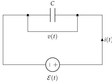
Here, we can model the voltage around the capacitor using the following differential equation:
